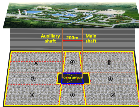
Fig. 12 Schematic diagram of the 3G N00 mining method of the AFR with non-pillars (He & Wang, 2019)
